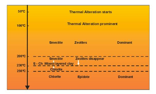
FIGURE 5: Alteration mineralogy and temperature
