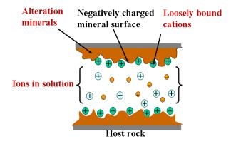
FIGURE 2: Conduction mechanisms
