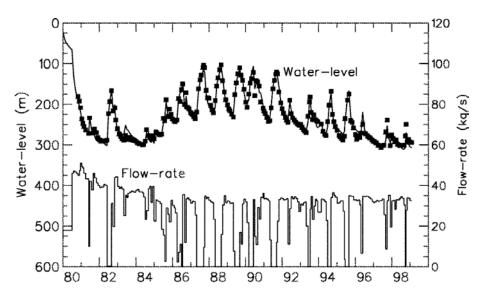
FIGURE 10: Production and water level history of the Ytri-Tjarnir low-temperature geothermal system in central N-Iceland 1980-1999. The water level history has been simulated by a lumped parameter model (squares = observed data, line = simulated data; Axelsson et al., 2005).
