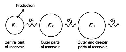
FIGURE 9: A 3-tank lumped ladder model commonly used to simulate geothermal systems (Axelsson et al., 2005)
