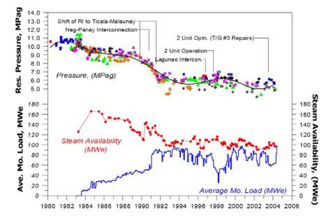
FIGURE 6: The production and pressure response history of the Palinpinion-1 volcanic geothermal system in The Philippines (Aqui et al., 2005)
