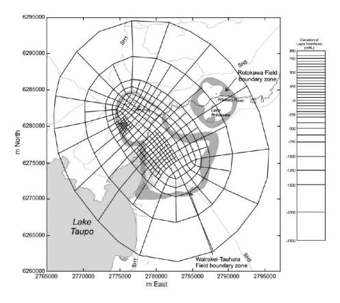
FIGURE 12: A horizontal and vertical sketch of the computational grid a recent numerical reservoir model of the Wairakei geothermal system in New Zealand (O'Sullivan et al., 2009)
