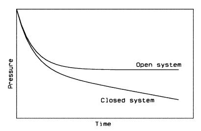
FIGURE 3: Schematic comparison of pressure decline in open (with recharge) or closed (with limited or no recharge) geothermal systems at a constant rate of production (Axelsson, 2008)
