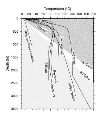
FIGURE 2: Formation temperature profiles for low-temperature systems in and around Reykjavík in SW-Iceland demonstrating the convective nature of the systems, through which heat has been transported from depth up to shallower levels (from Björnsson et al., 2000). Lighter shading denotes temperatures lower than to be expected from the regional gradient and darker shading the opposite.
