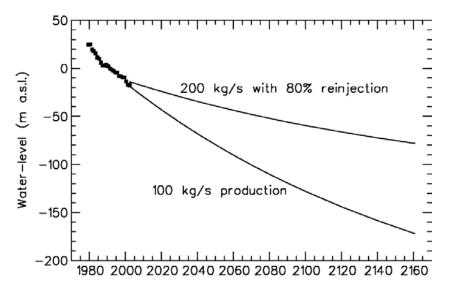
FIGURE 11: Predicted water level changes (pressure changes) in the Urban geothermal system under Beijing in China until 2160 for production scenarios with and without reinjection, averages of predictions calculated by a closed and an open lumped parameter model (Axelsson, 2010)
