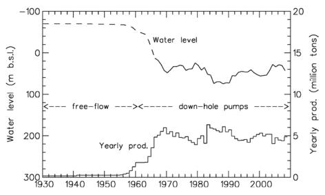
FIGURE 4: History of production and water level (pressure) response of the Laugarnes convective geothermal system in SW-Iceland from 1930 (Axelsson, 2012)
