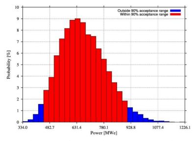
FIGURE 8: An example of the results of a volumetric resource assessment for the so-called "heavilyexplored part" of the Olkaria geothermal system in Kenya for a 50-year generation period (Axelsson et al., 2013). The Monte Carlo method was applied in the assessment. Note the great uncertainty in the results (electrical generation capacity) which arises from the uncertainty in key parameters.
