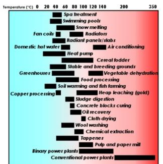
FIGURE 1: Lindal Diagram showing different applications of geothermal resources based on temperature
