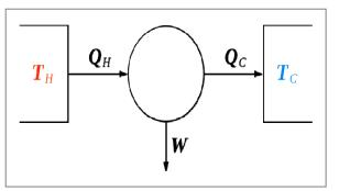
Figure 2: Thermal Cycle showing heat flow through an energy conversion system
