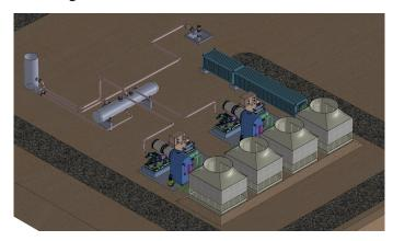
FIGURE 6: Typical layout of a wellhead generator installed by Green Energy Group in Olkaria, Kenya (Green Energy Group, 2011)
