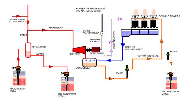
FIGURE 5: Processes of high temperature geothermal power plants
