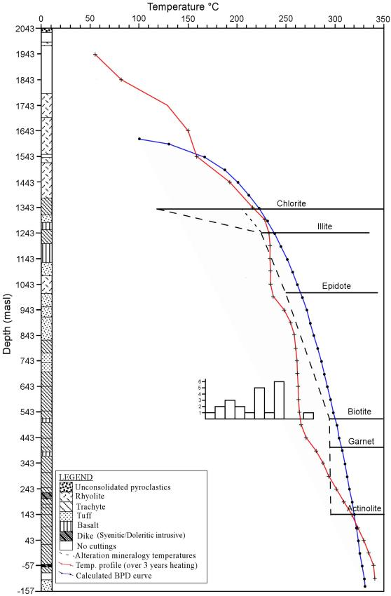
FIGURE 7: Plot of lithology and correlation between measured, interpreted hydrothermal alteration minerals and fluid inclusion temperatures with depth of well OW-903
