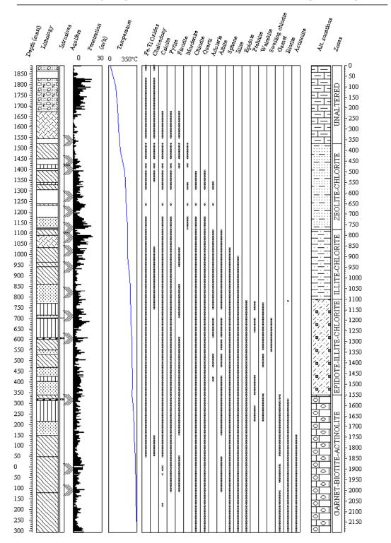
FIGURE 2: Lithology, distribution of hydrothermal alteration minerals and zonations in well OW-901
