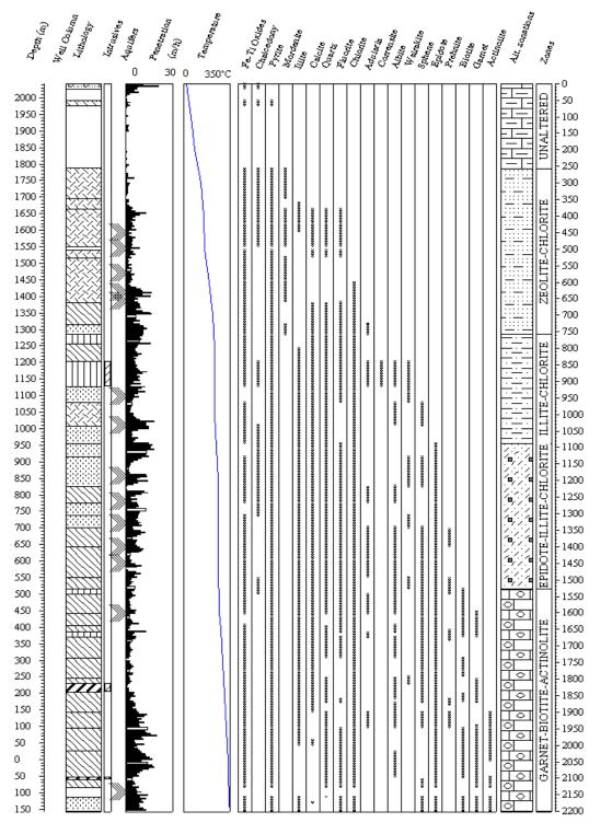
FIGURE 4: Lithology, distribution of hydrothermal alteration minerals and zonations in well OW-903
