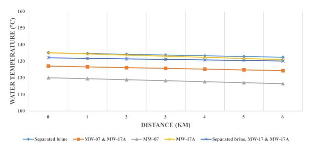
FIGURE 19: Temperature of hot water along a pipeline
