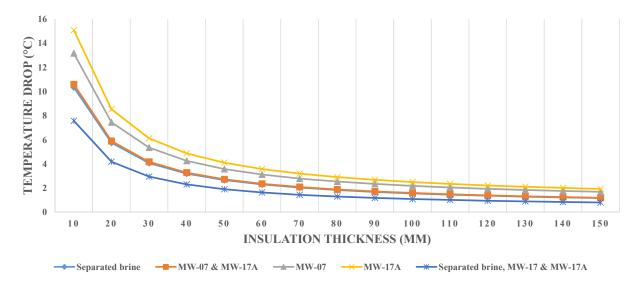
FIGURE 18: Temperature drop as a function of insulation thickness
