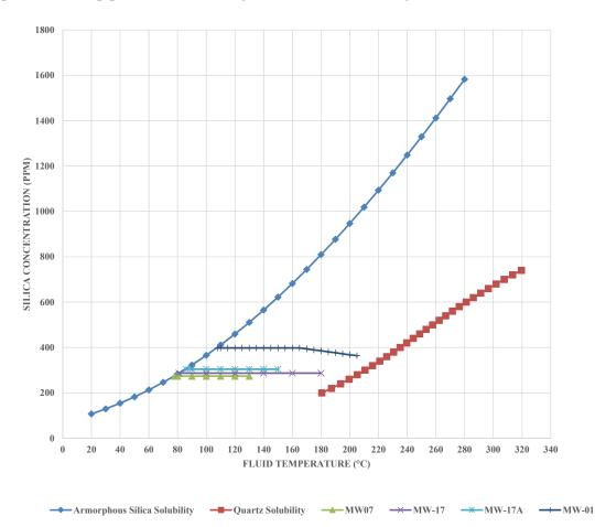
FIGURE 11: Silica solubility curves for fluids from selected wells in Menengai
