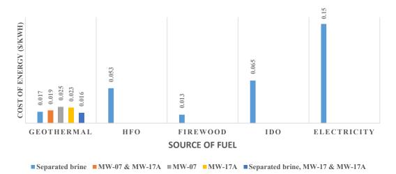
FIGURE 20: Comparison of the price of alternative sources of energy
