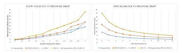
FIGURE 16: Pressure drop as a function of flow velocity and pipe diameter
