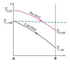
FIGURE 12: Counter current flow temperature profile (Haslego and Polley, 2002)
