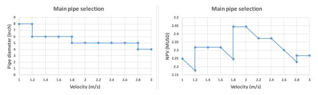
FIGURE 14: Sizing of a water pipeline
