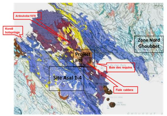
FIGURE 4: Geological map of the Assal Rift (Stieltjes, 1978); hyaloclastites are in orange, recent basalts in deep blue and violet. Early rift basalts (300.000 – 100.000 y.) are in pale blue; the stratoid series (3 to 1 My) is in very pale blue colour; lacustrine deposits (diatomite) in yellow
