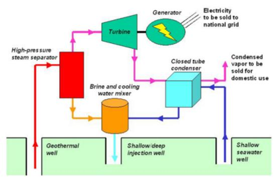
FIGURE 3: A conceptual design of a power plant proposed by Reykjavík Energy Invest, 2009 (Hjartarson et al., 2010)
