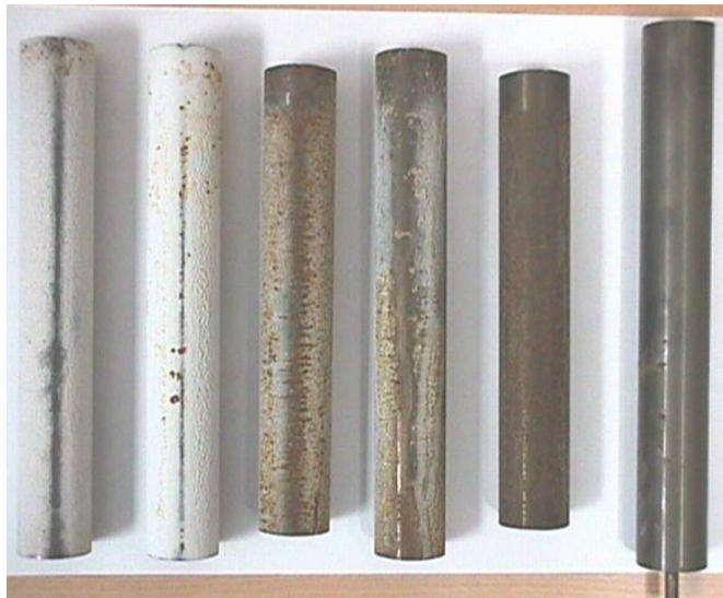
FIGURE 8: Silica scaling under controlled hydrodynamic and colloid particle size. From L to R: large particles - slow velocity, large particles - fast velocity, medium particles - low velocity, medium particles - fast velocity, small particles - low velocity and small particles - fast velocity
