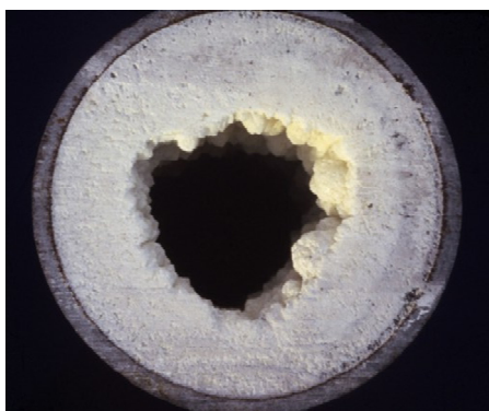
FIGURE 13: Calcite scaling in a 3” bore. This deposit formed in ~ 3 weeks
