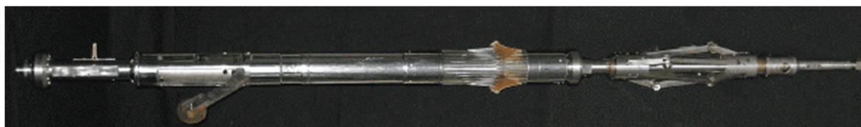
FIGURE 2: Photo of a 30-arm Multifinger caliper tool
