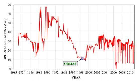
FIGURE 2: Power generation history of the Momotombo geothermal field (Porras, 2012)
