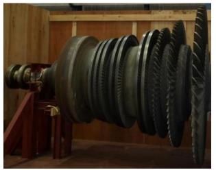
FIGURE 4: Steam turbine rotor
