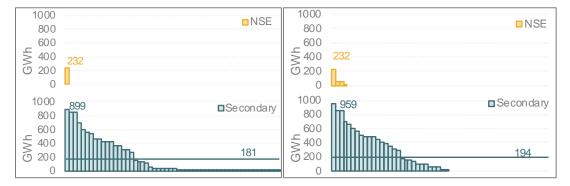
Figure 32: Curtailment levels by year 2030 under the Inter-regional reinforcement with wind (left) and without wind (right)
