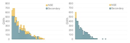
Figure 17: Total curtailments around Reykjavik before (left) and after (right) the reinforcement
