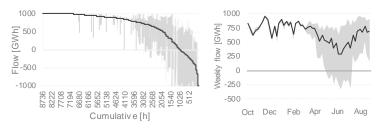
Figure 44: Energy flow through IceLink on an hourly (left) and weekly (right) basis (average level and range variation)
