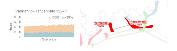
Figure 45: Number of hours in each year when the energy flow of the line connecting Varmahlið and Rangárvellir is at 100% (orange) and above 90% (blue) of its capacity limit
