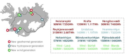
Figure 41: New generation investment (in bold) required in the IceLink case for the Inter-regional network reinforcement
