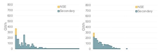
Figure 18: Total curtailments in the Reyðarfjörður industrial area before (left) and after (right) the reinforcement
