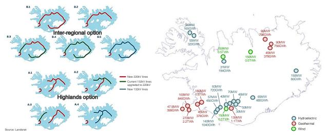
Figure 13: Alternatives in transmission (left side) and generation (right side) considered for achieving security of supply
