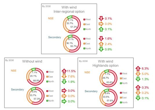
Figure 35: Curtailments per region under Inter-regional reinforcement with wind (top), under any reinforcement without wind (bottom left) and under the Highlands reinforcement with wind (bottom right) by year 2030f<sup>23</sup>
