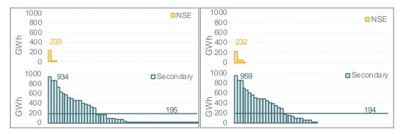
Figure 33: Curtailment levels by year 2030 under the Highlands reinforcement with wind (left) and without wind (right)
