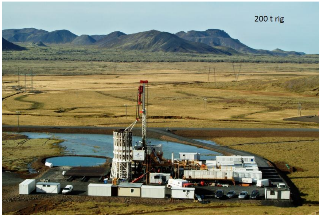
Fig. 4. A drilling rig on site at Hellisheiði (200 t hook load capacity). Photo Jarðboranir.
